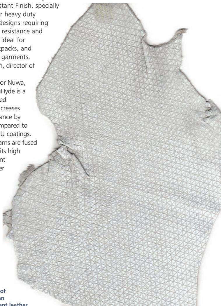
**Noticeable etched pattern on the surface of Pittards' Keratan abrasion-resistant leather.**
