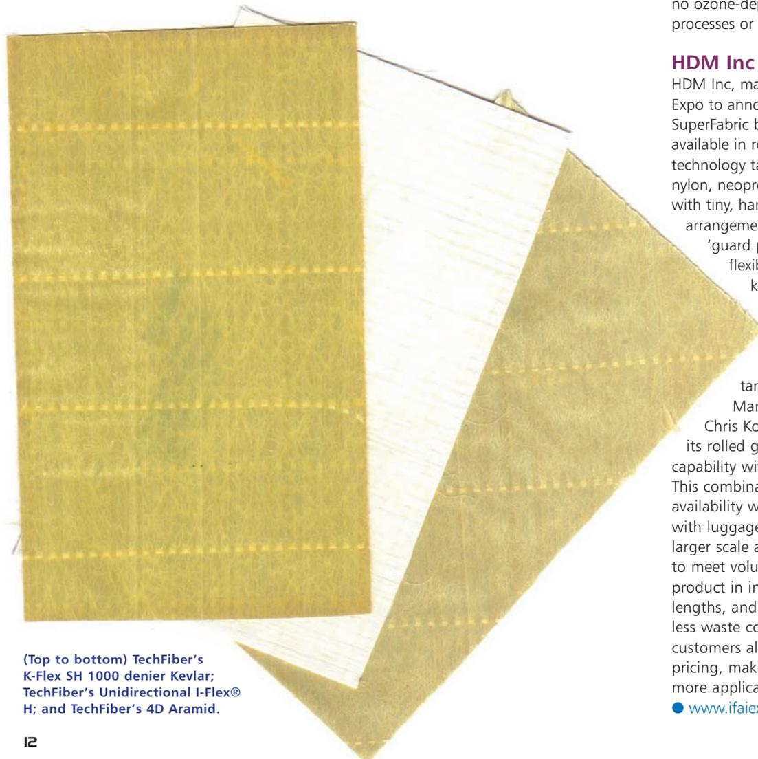
(Top to bottom) TechFiber's K-Flex SH 1000 denier Kevlar; TechFiber's Unidirectional I-Flex® H; and TechFiber's 4D Aramid.
