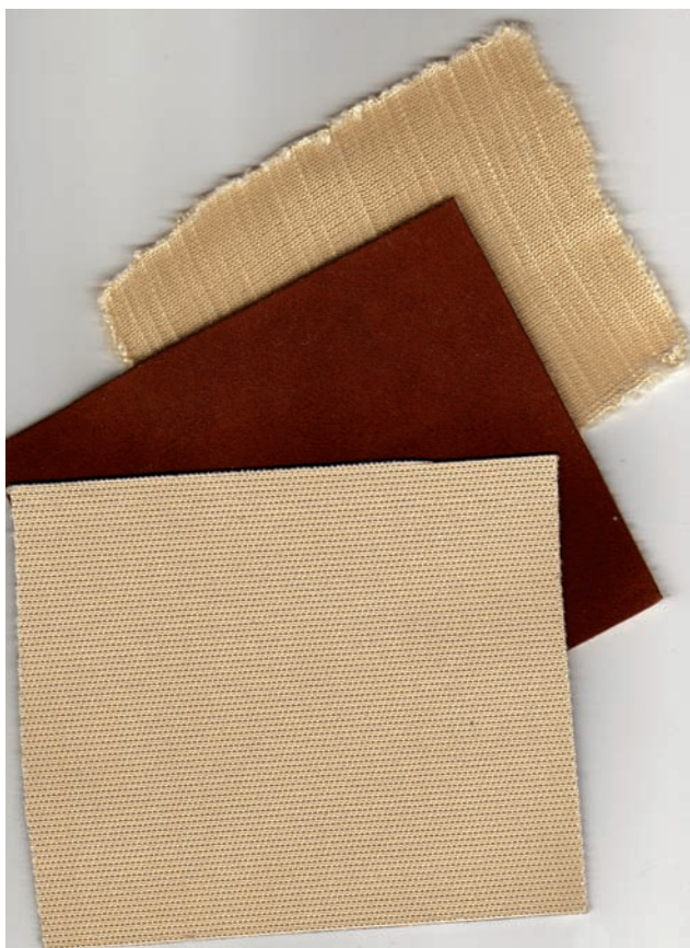
(Top) Vectran's new double knit interlock fabric; (centre) Vectran double knit interlock fabric bonded to the reverse side of Kuraray's Clarino leather; (bottom) the right side (the Kuraray Clarino leather side) of the Vectran interlock bonded fabric.
